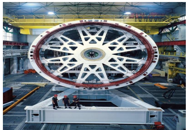
Fig.10. Example of a direct drive MW wind turbine generator
